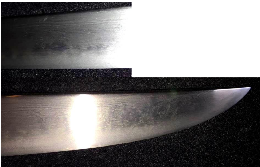
Figure 3 - These figures show the hada of the sword.
